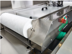
Closed-circuit tank with inclined filter
