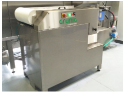
Closed- loop tank with inclined filter
