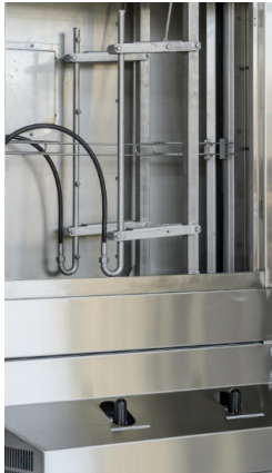
Oscillating nozzles on both screen sides
