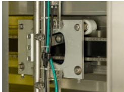
Spray carriage drive unit with sliding clutch
