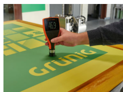
Measuring the layer thickness and surface roughness
